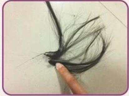
**Synthetic:**Burning smells like a burning plastic,there is a small flame,and feels viscous when it burns out.
