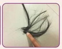
Synthetic:Burning smells like a burning plastic, there is a small flame, and feels viscous when it burns out.
