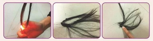
Synthetic:Burning smells like a burning plastic,there is a small flame,and feels viscous when it burns out.
